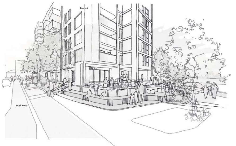
Sketch 5 illustrates the level change from Dock Road to the proposed café/restaurant, creating a raised, sheltered terrace that offers a safer and more comfortable seating area.
