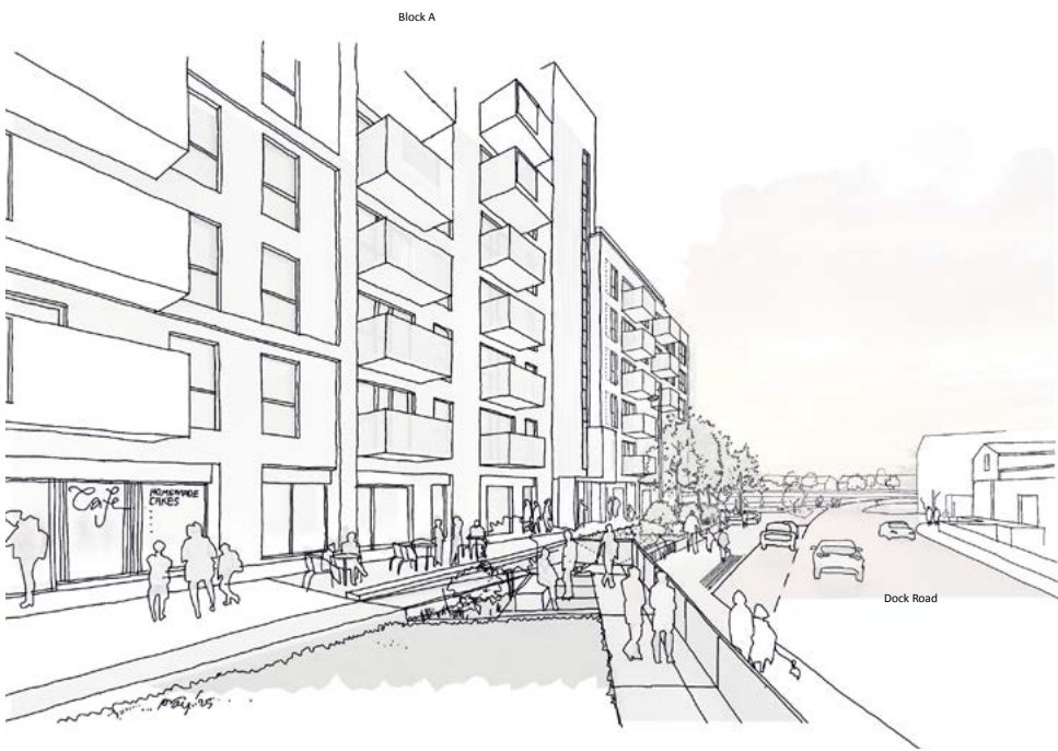
Sketch 1 shows the street elevation of Block A, featuring steps and ramp access from Dock Road to accommodate the level change.
