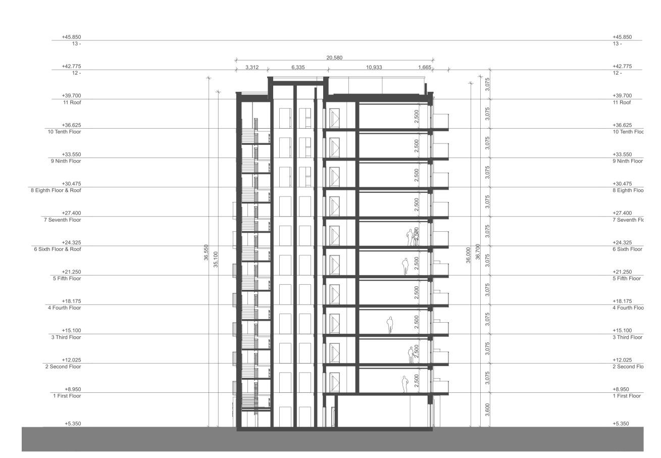
Section B-B SCALE:1:200 This drawing is the property of Altu Architects Ltd. It must not be copied or given to a third party without the permission of Altu Architects
